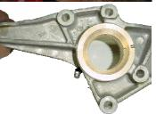
6 – Install bearings into the torsion bar tube.
